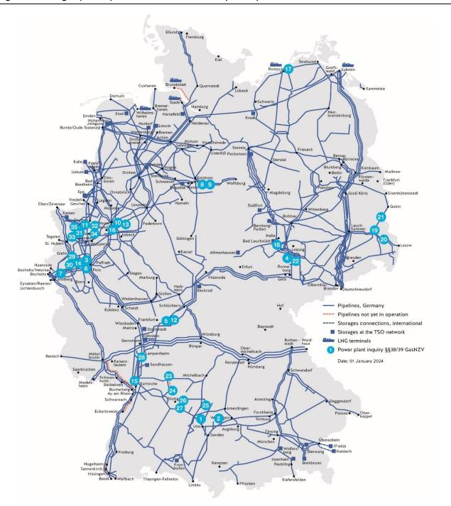
Source: Gas transmission system operators, schematic diagram
