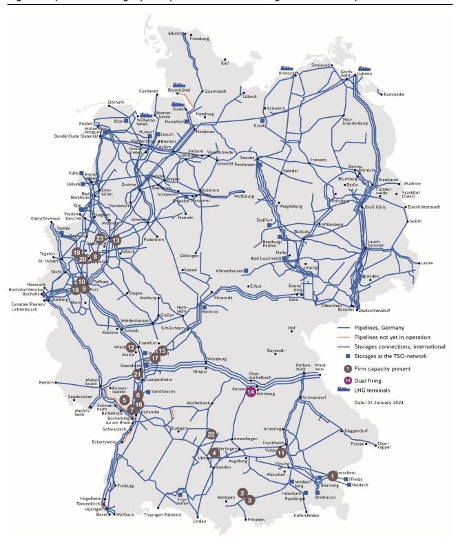
Figure 8: System-relevant gas power plants connected to the gas transmission system
