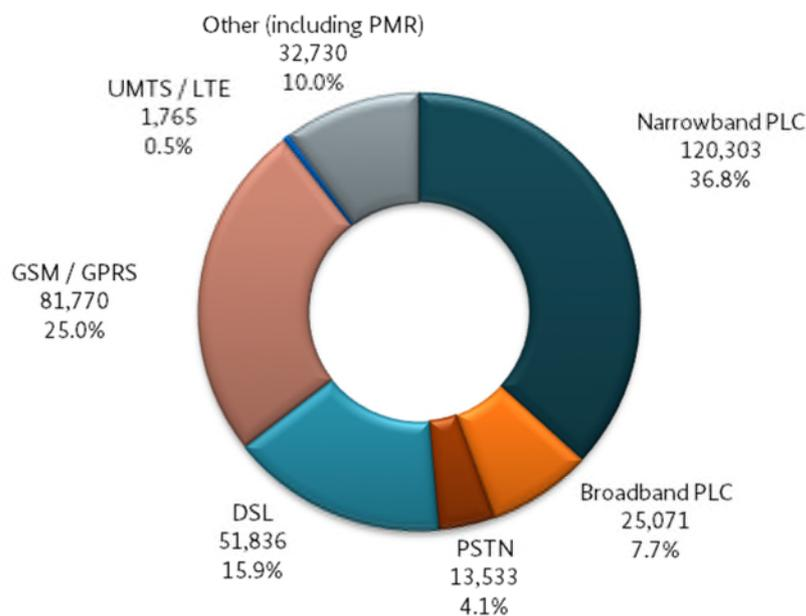
**Meter technology for interval-metered customers**
